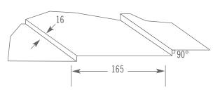
When ordering, it is necessary to specify the dimension from the end of the Profile sheet at eaves to the first batten or support.
