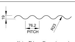
Note: This profile can be used for roof and wall cladding
