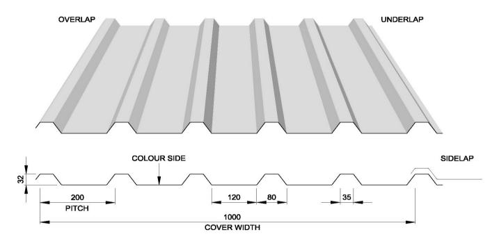
This section is also available with mini ribs in the troughs, Ref: TPP 1000-32 Forward.
